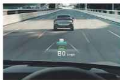
Augmented Reality Head-up Display Essential driving data displayed where you need it most.
