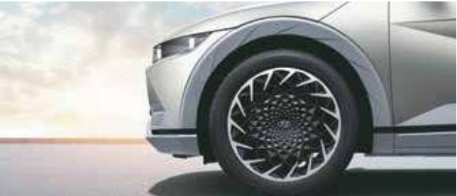
R20 (D=512.8 mm) Parametric pixel design alloy wheels
