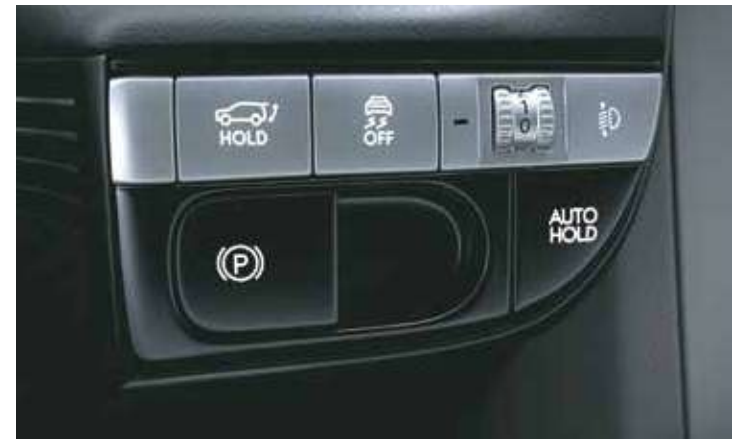
Electric parking brake (EPB)
