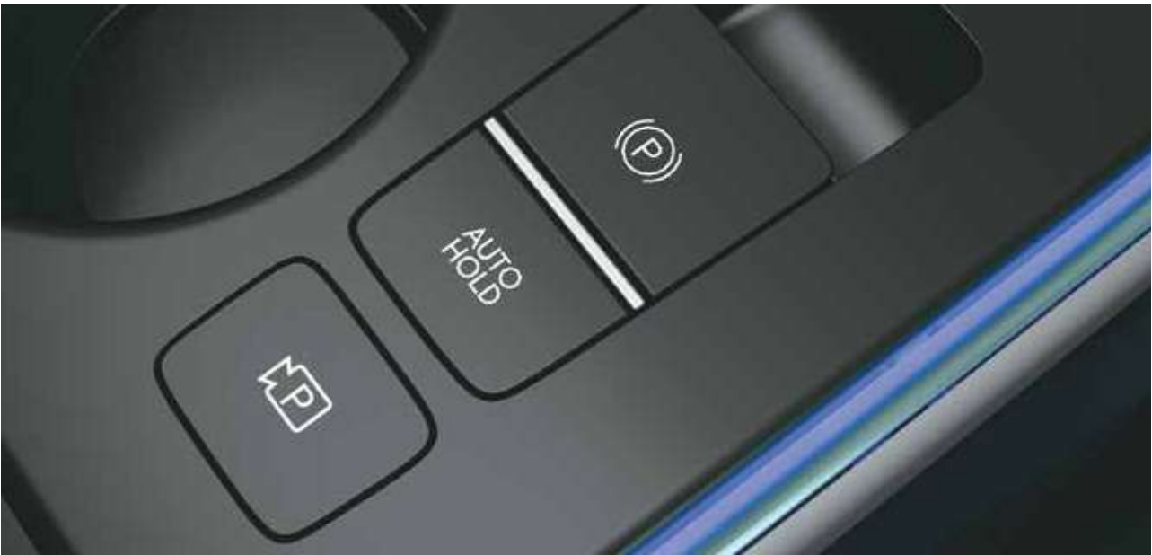
Electric parking brake with auto hold
